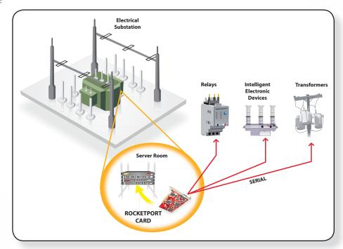
substation computer communicates to the central station by Ethernet across the WAN (Wide Area Network).
