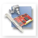
Conformal coating is a protective non-conductive dielectric layer that is applied onto the printed circuit board assembly to protect the electronic assembly from damage due to contamination, salt spray, moisture, fungus, dust, and corrosion caused by harsh or extreme environments.
